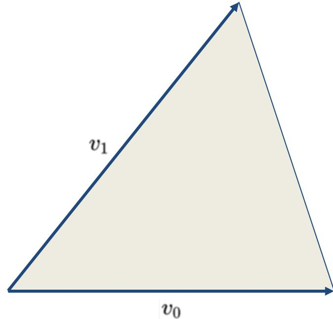
$$\text{area} = \frac{\|v_0 \times v_1\|}{2}$$
